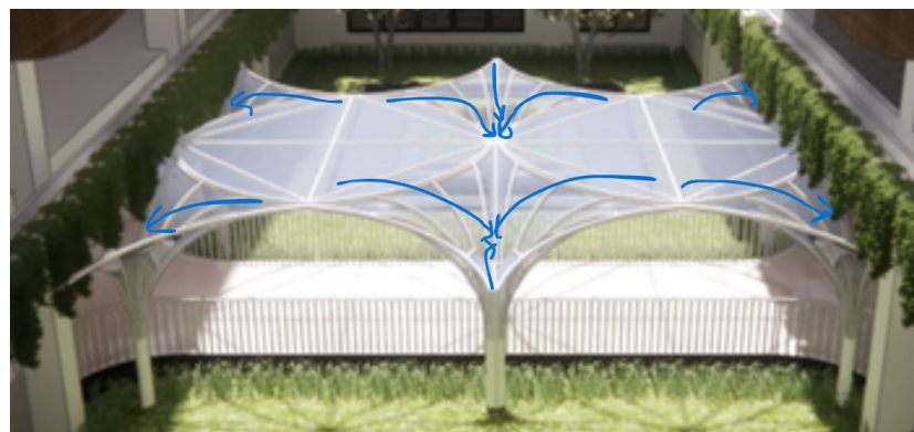
Gambar 7. Penerapan rainwater harvesting
