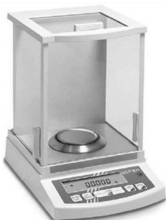
Gambar 2. Neraca Analitik KERN ABJ/ABS 220-4
