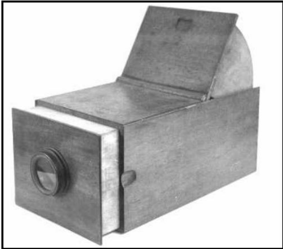
Gambar 1 Kamera Obscura (Sumber, www.physicskenyon.edu )
