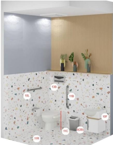
Fig 6. Accessible cubicle Multi-Stalled Enclosed Space Toilet
