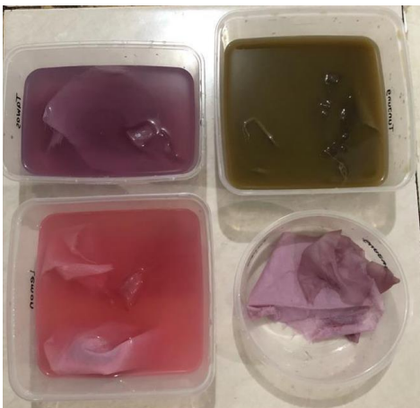
Fig. 2 Fixation Process, from upper left clockwise: Alum, FeSO 4 , without fixative, lemon juice. Source: Author's Documentation
