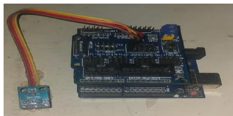
Figure 9. GY-30 BH1750 Sensor Design Results
